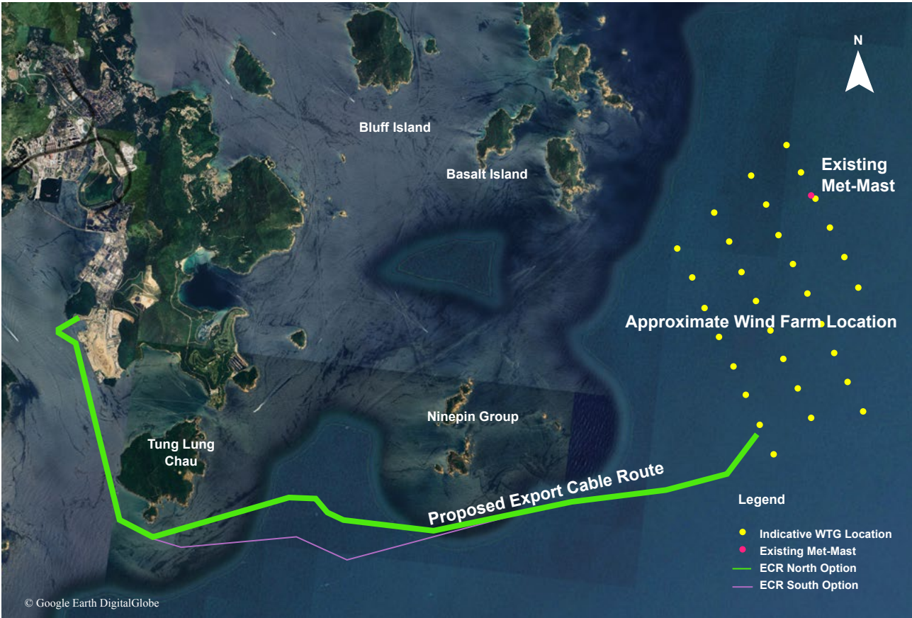
The proposed offshore wind farm project is located approximately 9km east of the Clearwater Bay peninsula and 5km east of East Ninepin Island in the south-eastern waters of Hong Kong, off the coast of Sai Kung district, in water depth of around 30m.
